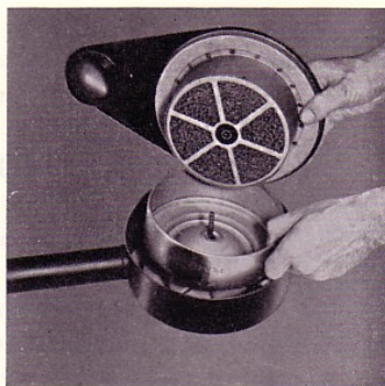
Fig. 21. Dismantling the air cleaner (B 16 A, B 18 A)
