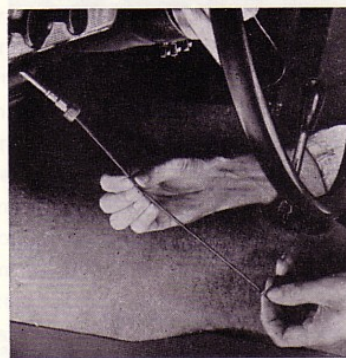
Fig. 28. Lubricating the drive cable
